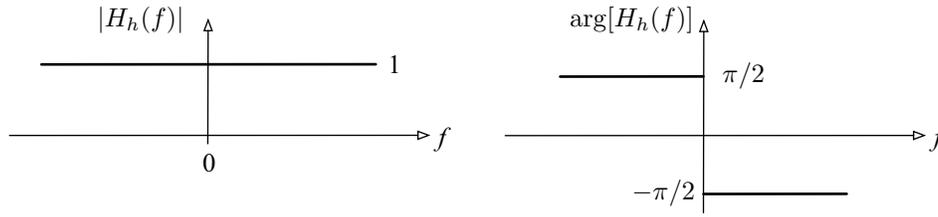
**Figure 5.24:** Magnitude and phase response functions of the Hilbert transformer.
