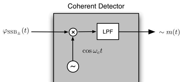
**Figure 5.28:** Demodulation of SSB signals using a coherent detector.
