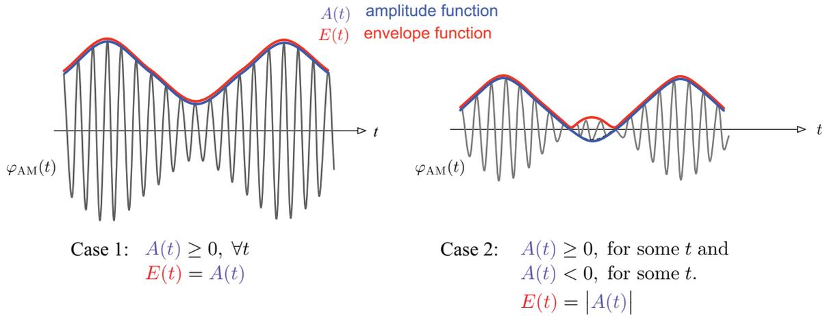
**Figure 5.12:** Amplitude and envelope functions of a modulated waveform.
