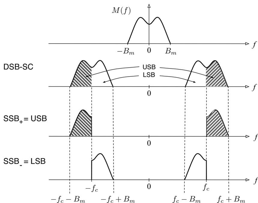
**Figure 5.22:** Spectra of DSB and SSB modulated waveforms.
