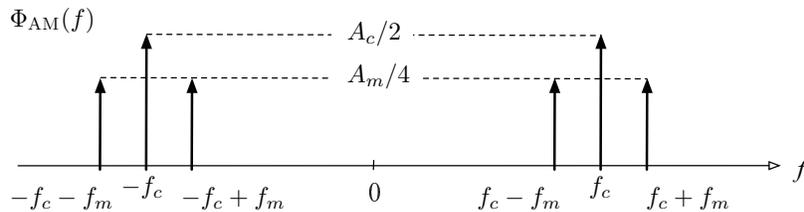
**Figure 5.16:**  $\Phi_{\text{AM}}(f)$  resulting from single-tone amplitude modulation.
