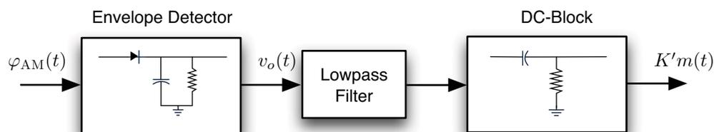
**Figure 5.20:** AM signal demodulation using envelope detection.
