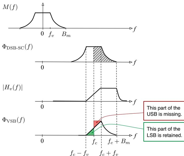
**Figure 5.30:** Spectra of the signals encountered during VSB signal generation based on selective filtering.
