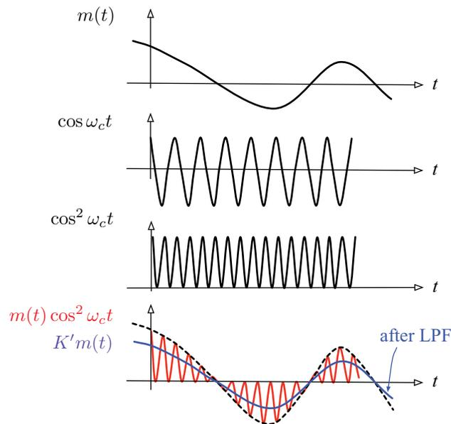
**Figure 5.6:** Time-domain waveforms at the demodulator.
