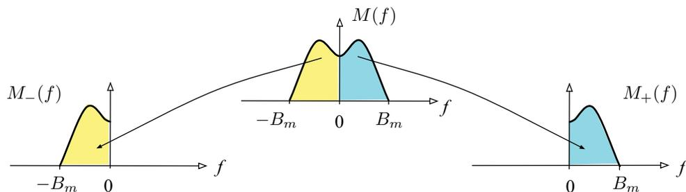
**Figure 5.23:** Single sideband spectra  $M_+(f)$  and  $M_-(f)$  generated from  $M(f)$ .
