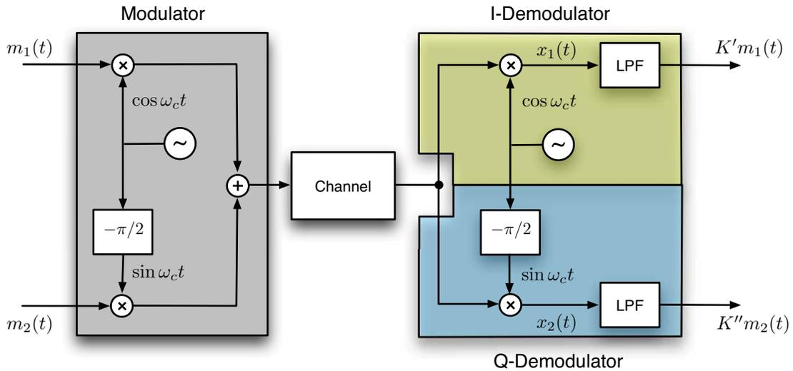
Figure 5.21: QAM modulator and demodulator.
