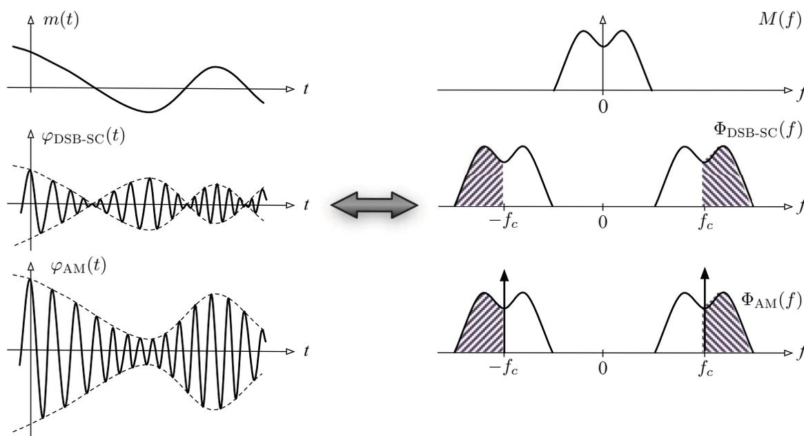
**Figure 5.11:** Time-domain waveform and spectrum comparison for DSB-SC and AM signals.
