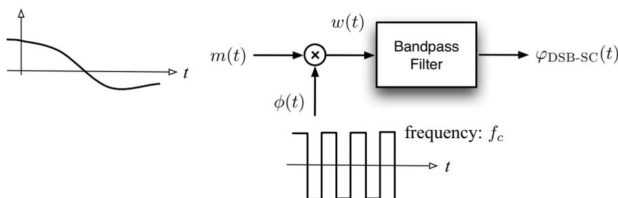
**Figure 5.8:** DSB-SC AM signal generation using a switching modulator.
