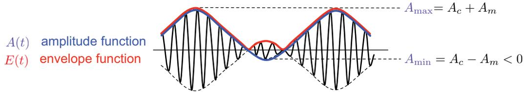
**Figure 5.15:** Modulated waveform for  $\mu = A_m/A_c > 1$ .
