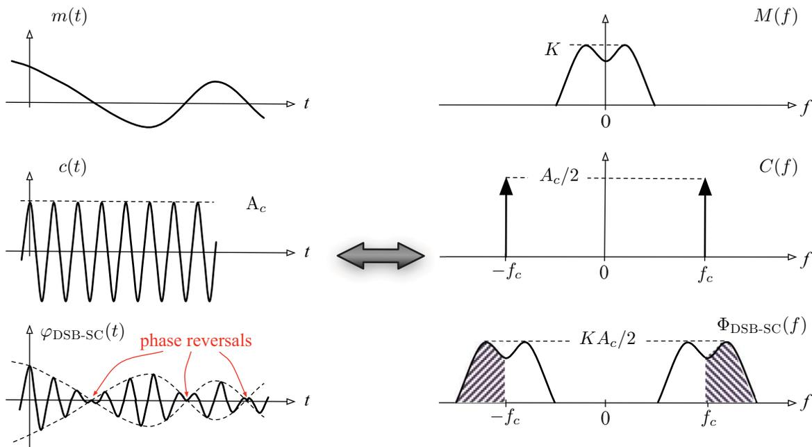
**Figure 5.3:** DSB-SC amplitude modulation.
