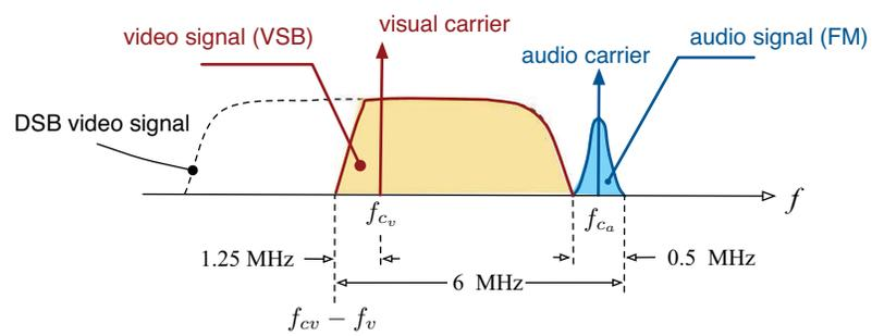
**Figure 5.33:** Spectrum of a typical composite TV signal ( $f_{c_v}$  : visual carrier,  $f_{c_a}$  : audio carrier such that  $f_{c_a} = f_{c_v} + 4.5$  MHz).
