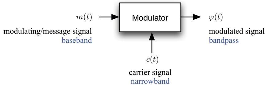
**Figure 5.1:** The modulation process.
