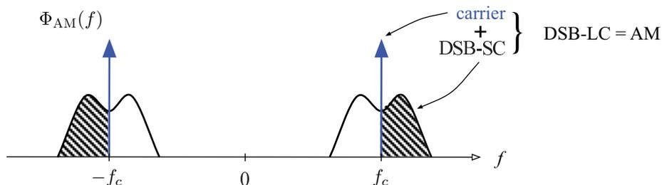
**Figure 5.10:** Spectrum of an DSB-LC/AM signal.
