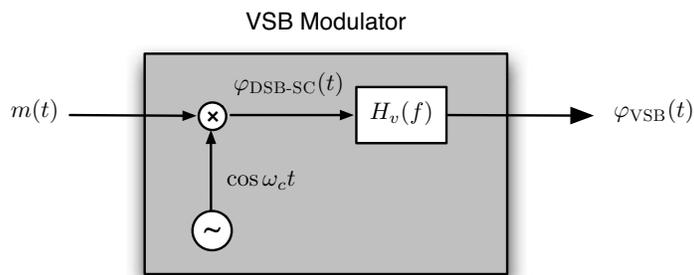
**Figure 5.29:** VSB signal generation using filtering.
