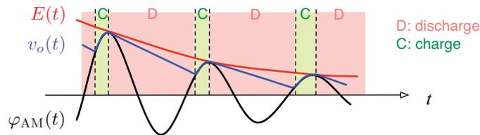
**Figure 5.18:** Charging and discharging of the capacitor in the envelope detector.
