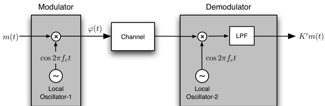
**Figure 5.5:** Generation and demodulation of DSB-SC amplitude modulated signals.
