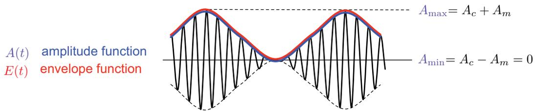
**Figure 5.14:** Modulated waveform for  $\mu = A_m/A_c = 1$ .
