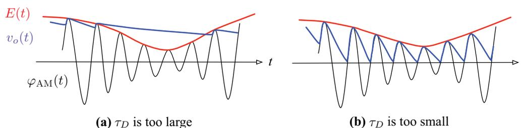
**Figure 5.19:** Envelope detector output: (a)  $\tau_D$  too large, (a)  $\tau_D$  too small.
