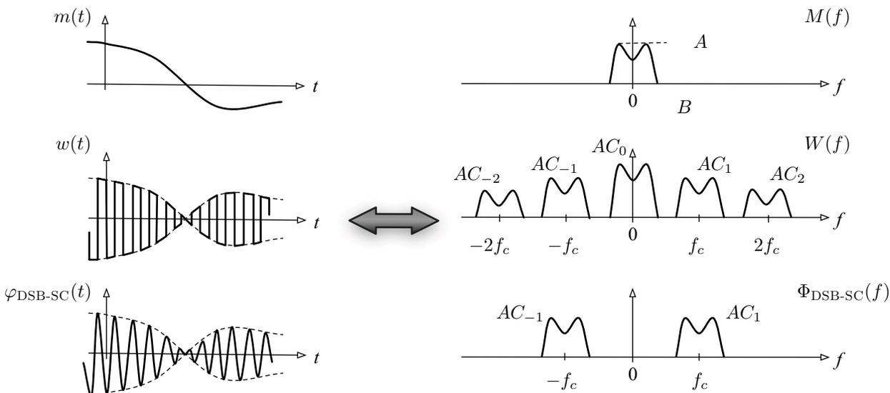
**Figure 5.9:** Time-domain waveforms and their spectra encountered in the switching modulator.
