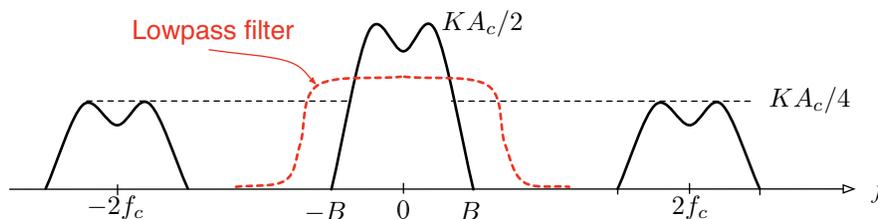
**Figure 5.4:** Spectrum of  $\varphi_{\text{DSB-SC}}(t) \cos \omega_c t$  and the recovery of  $m(t)$ .
