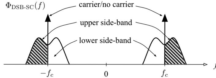
**Figure 5.2:** Elements of the spectrum of a modulated waveform.
