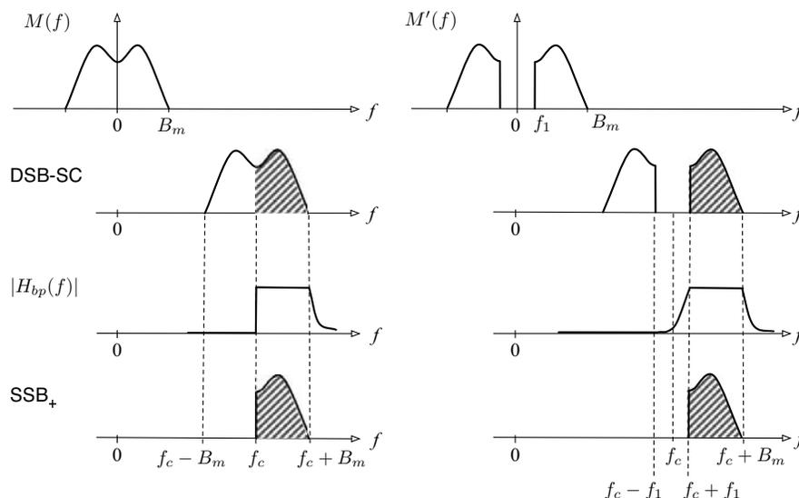
**Figure 5.26:** Generating a  $SSB_+$  signal from a DSB-SC signal using the selective filtering method based on (a)  $m(t)$  with low-frequency content and (b)  $m'(t)$  with a low-frequency hole.
