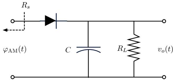
**Figure 5.17:** The envelope detector ( $R_L$  : load resistance,  $R_s$  : source resistance).
