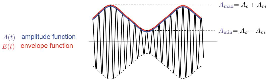
**Figure 5.13:** Modulated waveform for  $\mu = A_m/A_c < 1$ .
