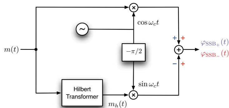
**Figure 5.27:** Generating SSB signals using the phase-shift method.
