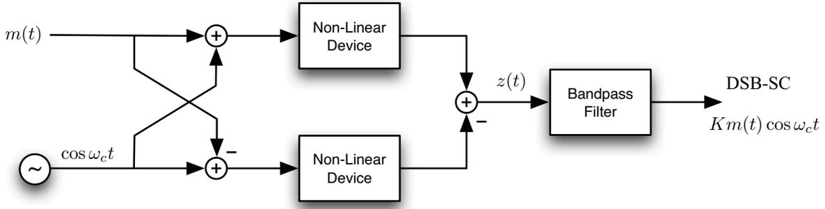
Figure 5.7: AM signal generation using non-linear modulator.
