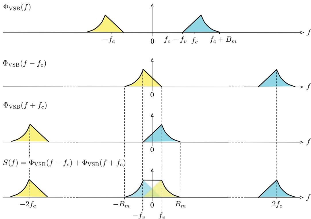
**Figure 5.31:** Demodulation of VSB modulated waveforms using a coherent detector.
