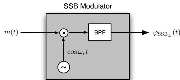
**Figure 5.25:** SSB signal generation using the selective filtering method.
